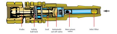
Quick release couplings make the connecting and disconnecting of hoses and regulators easy and quick. Safety is improved by incorporating non-return valves to prevent gases backfeeding and causing flashbacks.
